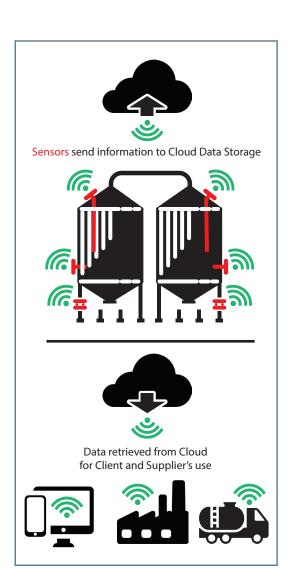
Silo Telemetry is the ability to remotely realise the content of a silo or vessel using the internet and mobile networks.
